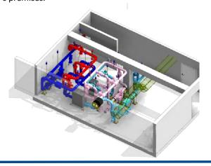
As part of the detailed design, a 3D model of the heat exchanger station is being worked up, along with detailed design of piping and components, risk assessment, etc.
